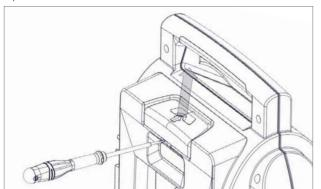
2. Replace with a new release button. Pay attention that the two springs are positioned in the guide of the release button.
