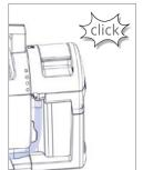
13. Check that the clip **1** of the canister lid is correctly attached to the support of the canister system.
