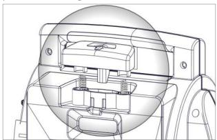
3. Press the release button downwards until it engages.
